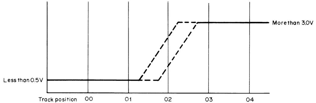
Adjust so that the level of the sensor output changes between track 01 (Low level) and track 03 (High level)
