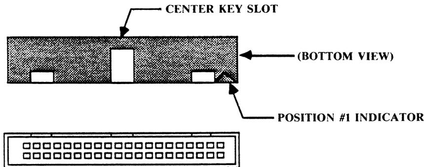
FIGURE 2 — AT-BUS INTERFACE CONNECTOR (J2)
